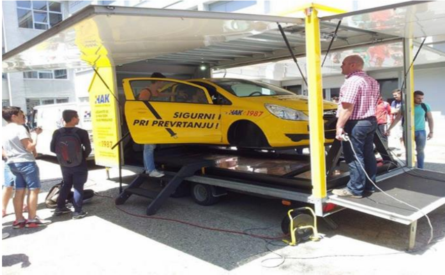
Figure 7. Overturning simulator - the role of seat belts
